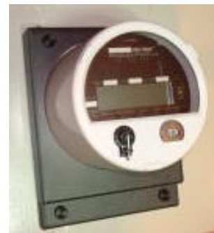
4. Installed with meter & cover
